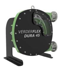
Verderflex positive displacement pumps are suitable to transfer a large variety of fluids. The liquid is totally contained within a flexible hose or tube fitted inside the pump casing. The hose or tube is the pump's only consumable part. All Verderflex pumps can be used in hygienic applications thanks to several food grade hoses and tubing.
